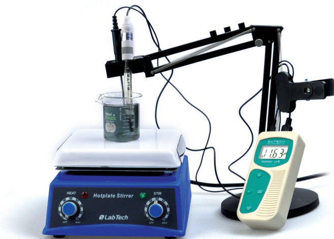
An experiment measuring ORP and pH while stirring
